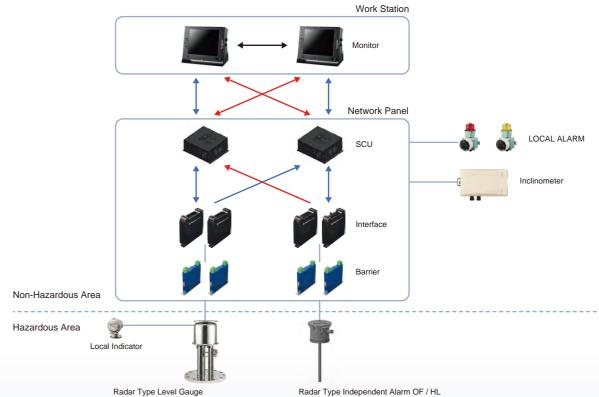
Radar Type Level Gauge - Level Gauge (Primary / Secondary)
