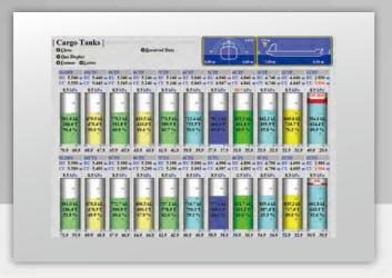
The tank monitoring software provides operators with an easy-to-understand graphic display of conditions in cargo, ballast and service tanks. Through this interface, operators can easily see current conditions for all tanks, as well as get detailed information from specific tanks as needed. The software also allows operators to set various parameters, such as type of cargo and variable alarm points.
